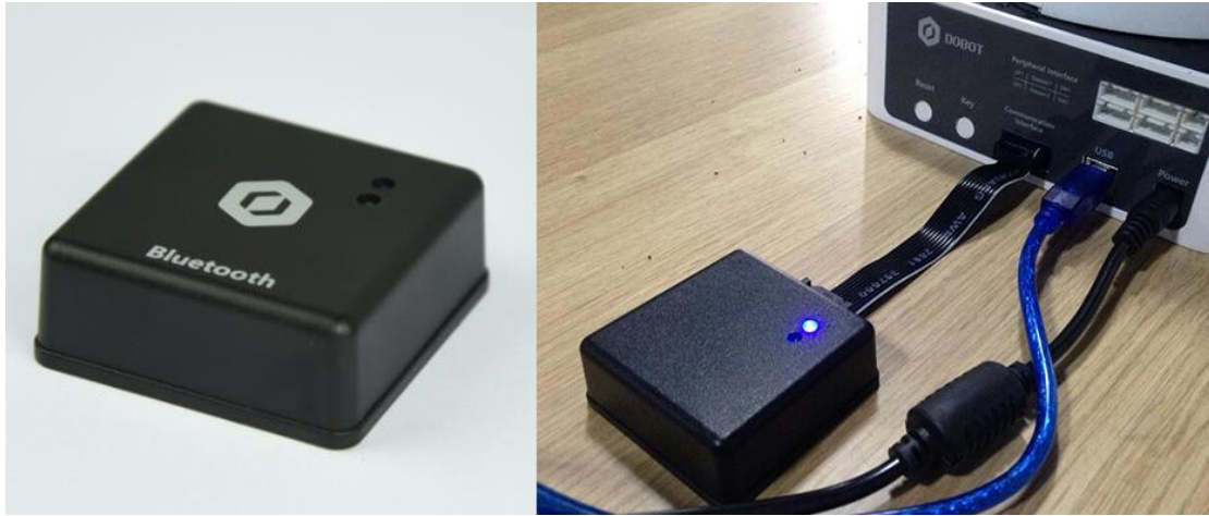
Figure 8.1 Bluetooth module installation
